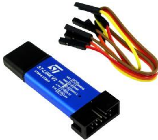
Figure (2-10) 8-STLINK STM8 STM32 Programmer
